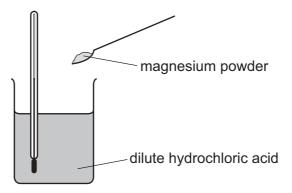
Thermometer reading before adding magnesium powder = 20.6 °C
