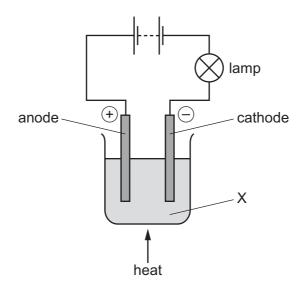
A brown gas is produced at the anode and a grey metal is produced at the cathode.
